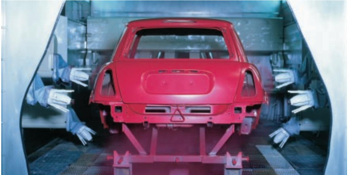
Mini production, base coat application, Oxford Plant
