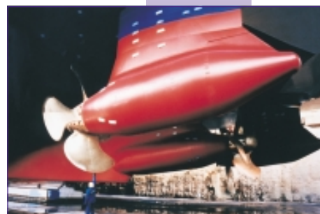
Azipod® power range starts at 400 kW and reaches 38 MW.
